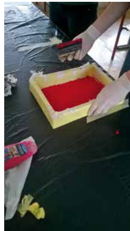
GRGO PETROV GRAFIČKE TEHNIKE / GRAPHIC TECHNIQUES MENTOR: Mario Petrak — Proces otiskivanja sitotiska / Screen Printing Process
